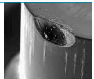
Edge chipping due to cyclic plastic deformation 由於循環塑性變型造成的邊緣崩角
