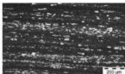
圖 12% 之常規 鋼微合金相組織 Micro structure of conventional 12% chromium steel
